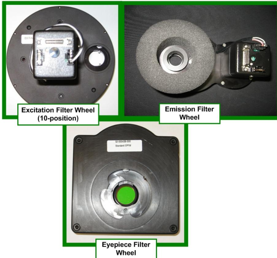
A filter wheel module includes the Excitation, Emission, and Eyepiece filter wheels and can support up to six filter pairs.
