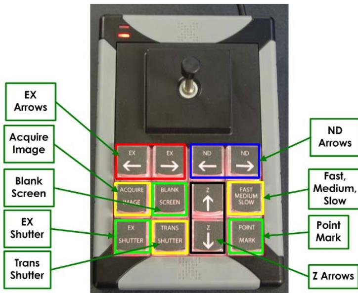
Figure 3.1 Key controls on the 12-key Keypad
