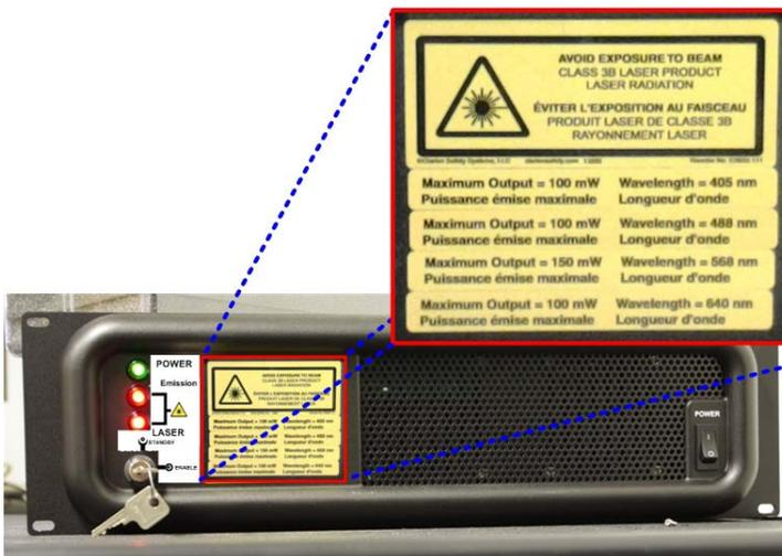
Laser Source Chassis Laser Safety Label Locations
