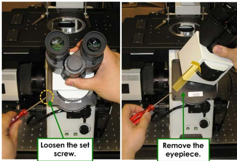
4. Loosen the set screw that holds the Eyepiece filter wheel to the beveled mount on the stand and remove the Eyepiece filter wheel.
