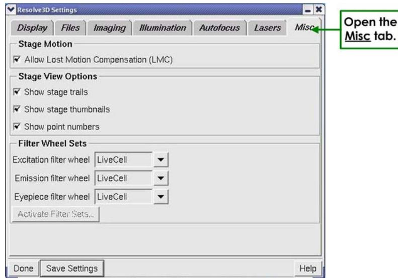
5. Select the newly installed Excitation, Emission, and Eyepiece filter wheels in their respective fields in the **Misc** tab.
