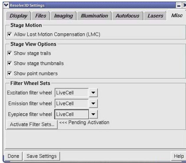
2. Verify that the **Excitation**, **Emission**, and **Eyepiece** filter wheel fields all display the expected and identical filter wheel module name (if any of the names are different, you may need to select or replace one or more of the filter wheels; see *Changing Filter Wheel Modules* on Page 9.4).
