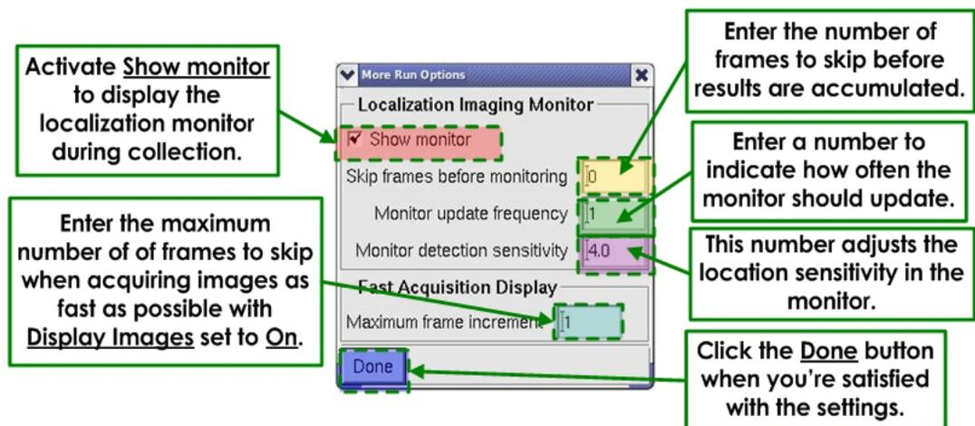
8. From the More Run Options window, activate the **Show monitor** check box to display the Localization Imaging Monitor during the collection process.
