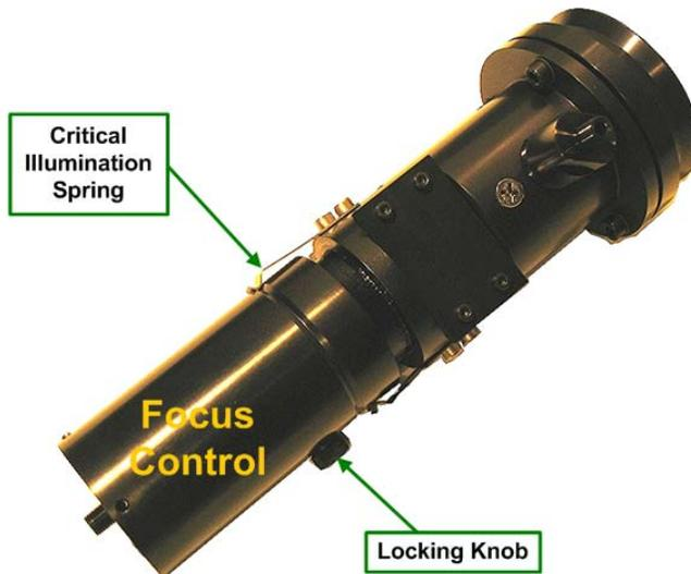
The FOM in Critical Illumination position, the Focus Control is extended so that the Critical Spring is in the groove.
