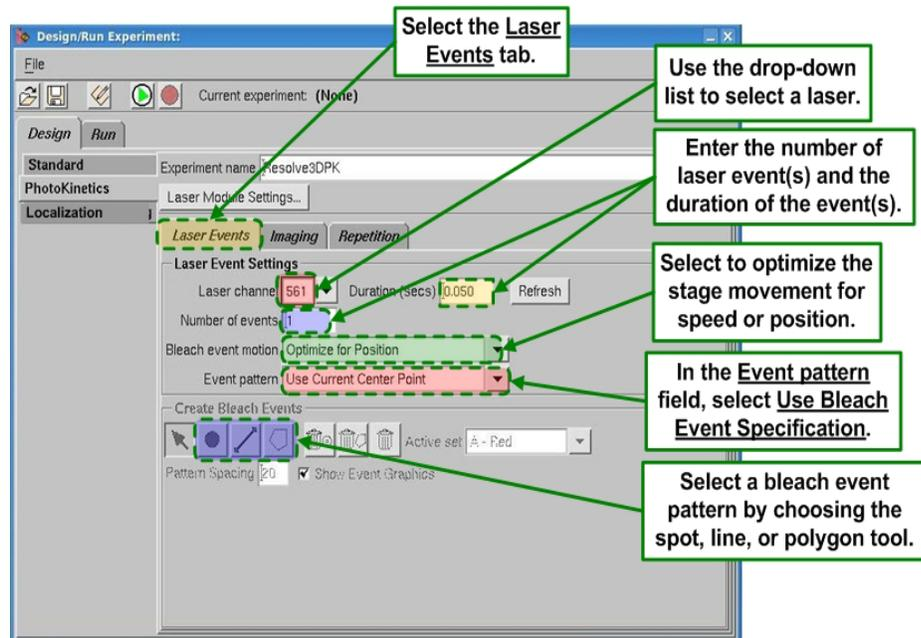
4. To generate multiple bleach events, the stage moves the sample to the site of laser activity. You can optimize this motion for either speed or position. When **Optimize for Position** is selected, the stage goes through an LMC (Lost Motion Compensation) move to achieve the most accurate position. This move takes more time than when **Optimize for Speed** is selected.
