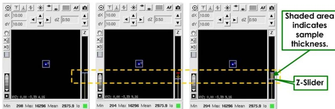
Use the Z slider to find the top and bottom of a sample. The sample thickness is indicated by the wide line on the Z slider (shown on the right image).
