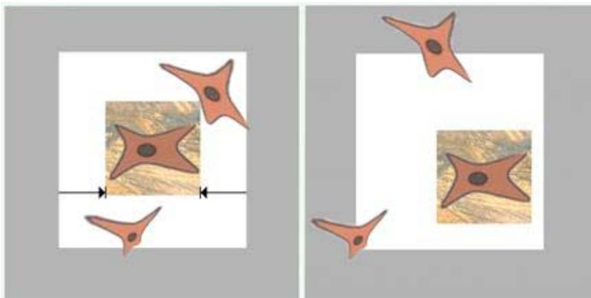
In the first image, the width of the ROI is defined as 50% of the width of the field of view. In the second image, the stage has moved to keep the cell of interest within the ROI. Perimeter cells have also moved, almost entirely out of the field.
