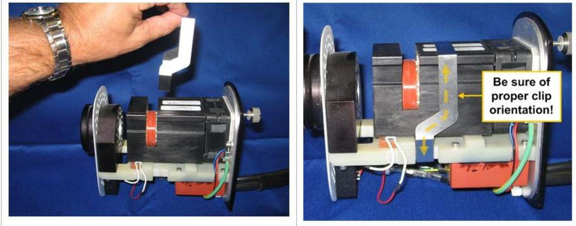
10. Gently slide the internal lamp mechanism into place within the lamp housing.
