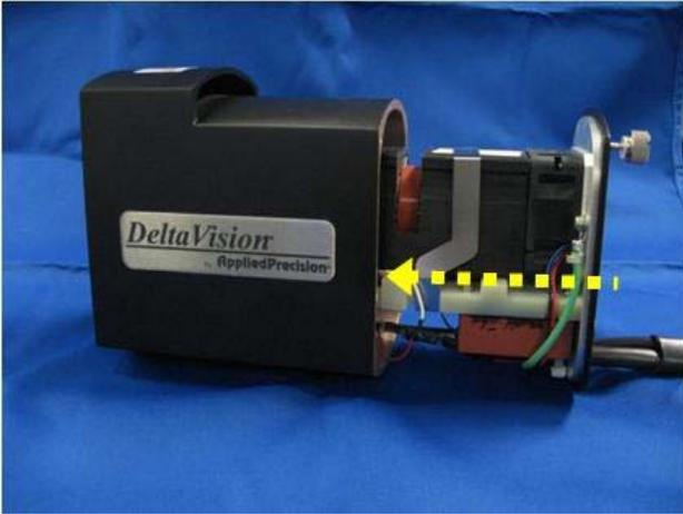
11. Tighten the two thumb screws on the end of the lamp housing.
