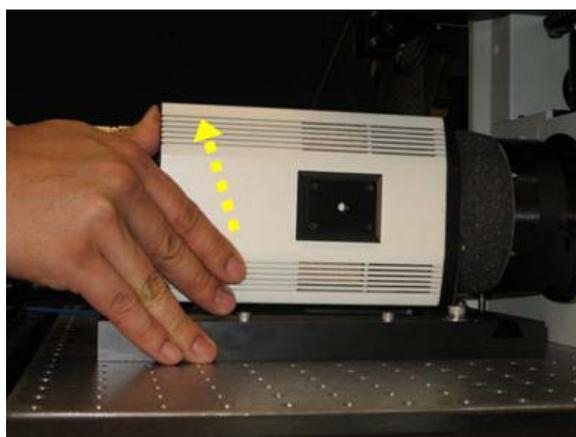
3. Remove the other camera from the spare camera tray and set it aside. Place the camera that you just removed on the spare camera tray.
