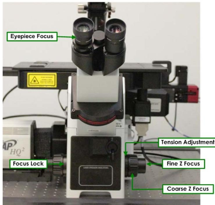
**Eyepiece Focus** – Use the Eyepiece Focus (on the left ocular) to adjust focus between the two oculars.
