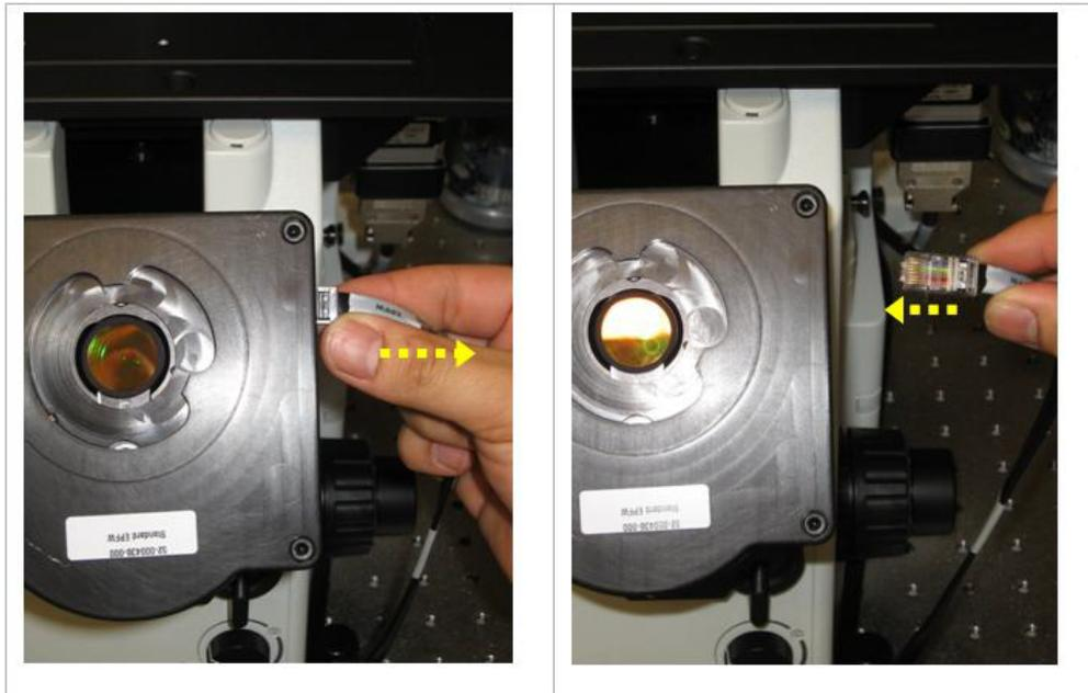
Note that it is not necessary to remove the oculars before plugging or unplugging the Eyepiece filter wheel.
