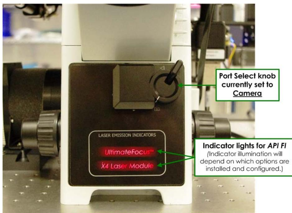
The port selector knob and the UltimateFocus and X4 Laser Module indicator lights are shown on the front of the DeltaVision microscope.
