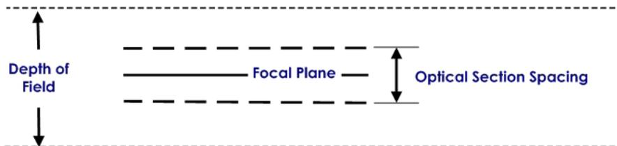
The Optical section spacing specifies the upper and lower boundaries for which information is collected. It is centered on the focal plane and includes the information above and below that plane.
