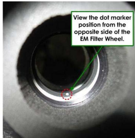
13. Reassemble the Emission Filter Wheel and reinstall the unit back onto the microscope. Adjust the Filter Wheel Support Screw so that the Emission Filter Wheel rests on the screw at maximum extinction as observed through the EM filter.
