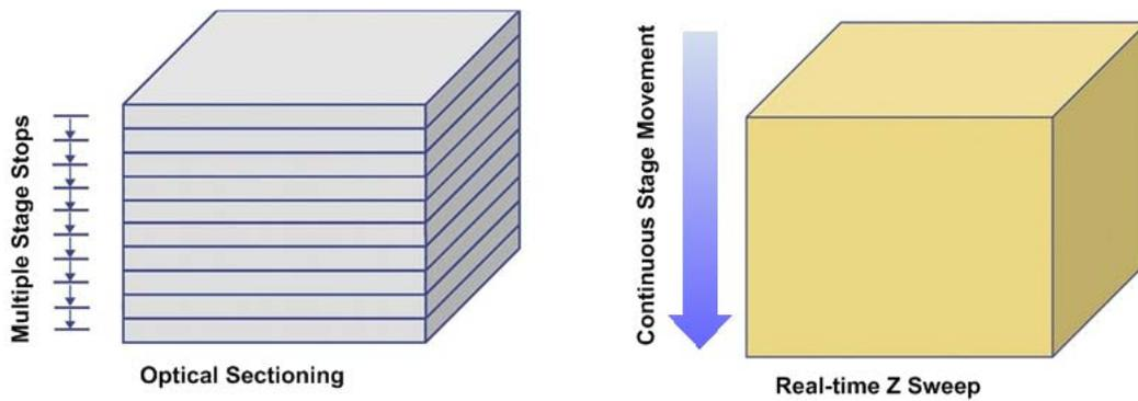
Instead of acquiring multiple images, Real-Time Z Sweep acquires one image during a continuous stage movement and instantly creates a 2D Z Projection.
