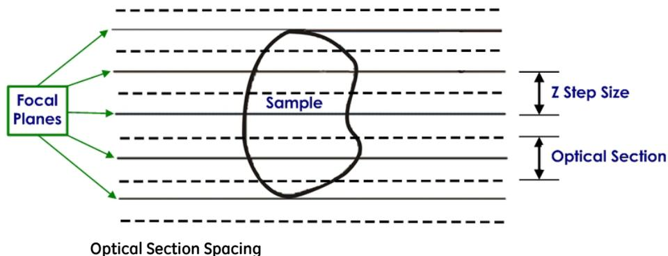
For example, the standard step size for a 1.42 NA lens is 0.2  $\mu\text{m}$ , although other step sizes are usually fine. Due to the inherent Z resolution of a 1.42 NA lens, there is little need to take steps finer than 0.1  $\mu\text{m}$ .
