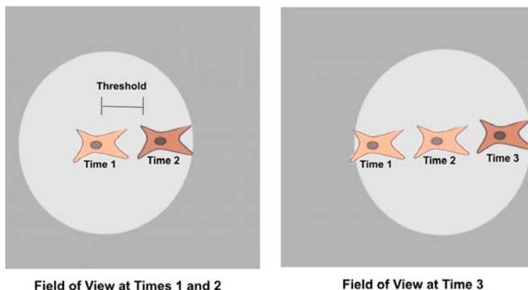
Cell tracking lags cell movement. Cell movement exceeds the threshold between Time Points 1 and 2 (left). In response, *DeltaVision* moves the stage so that it is centered on the cell position at Time Point 2. The stage is at this position when Time Point 3 is acquired (right).
