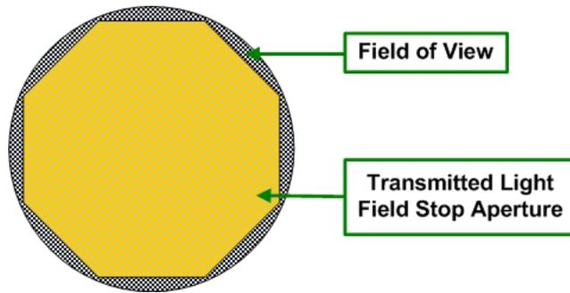
If you cannot see the entire iris while moving the Condenser Focus Knob, it may be necessary to alter the centering before you are able to focus on the edges of the iris.
