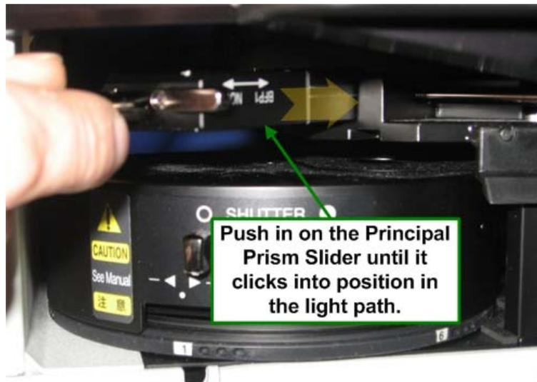
The Principal Prism Slider has two positions: **Normal** and **BFP1** (as shown below). The selected position will depend on the type of objective being used. If you are unsure, check the objective. It will say **BFP1** if that is the correct position.
