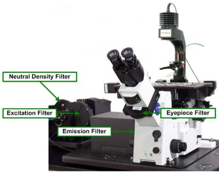
*DeltaVision* provides several different types of filters for controlling the fluorescent light path:
