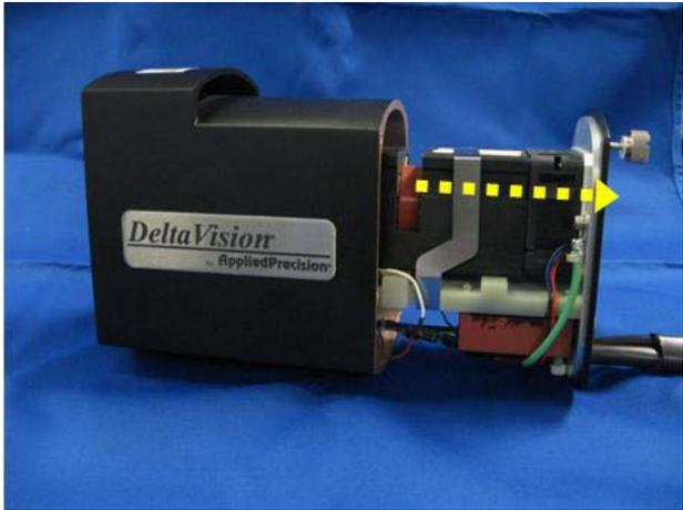
6. Remove the center clip from the internal lamp mechanism as shown.
