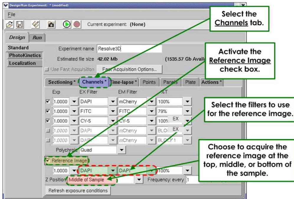
This experiment specifies using the DAPI and Cy-5 filters to acquire images of each section and using the transmitted light to acquire a reference image using the DAPI filter in the middle of the sample.
