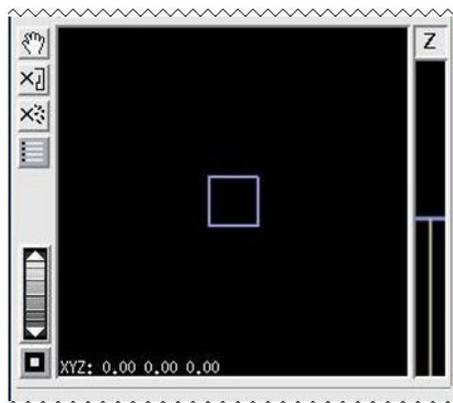
The blue box represents the current stage location. Drag the box to move the stage in X and Y.
