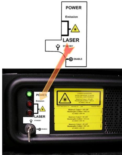
**Laser Module Key Switch Label Location**
