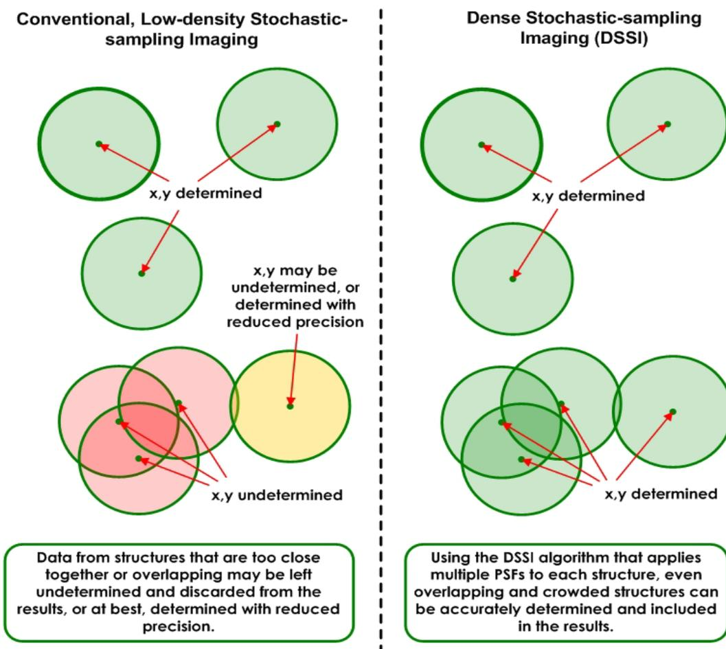
Rather than discarding data produced from overlapping fluorophores, the algorithms used in DSSI have the ability to examine the data more closely by iteratively attempting to fit multiple Gaussians to overlapping or densely labeled fluorophores.
