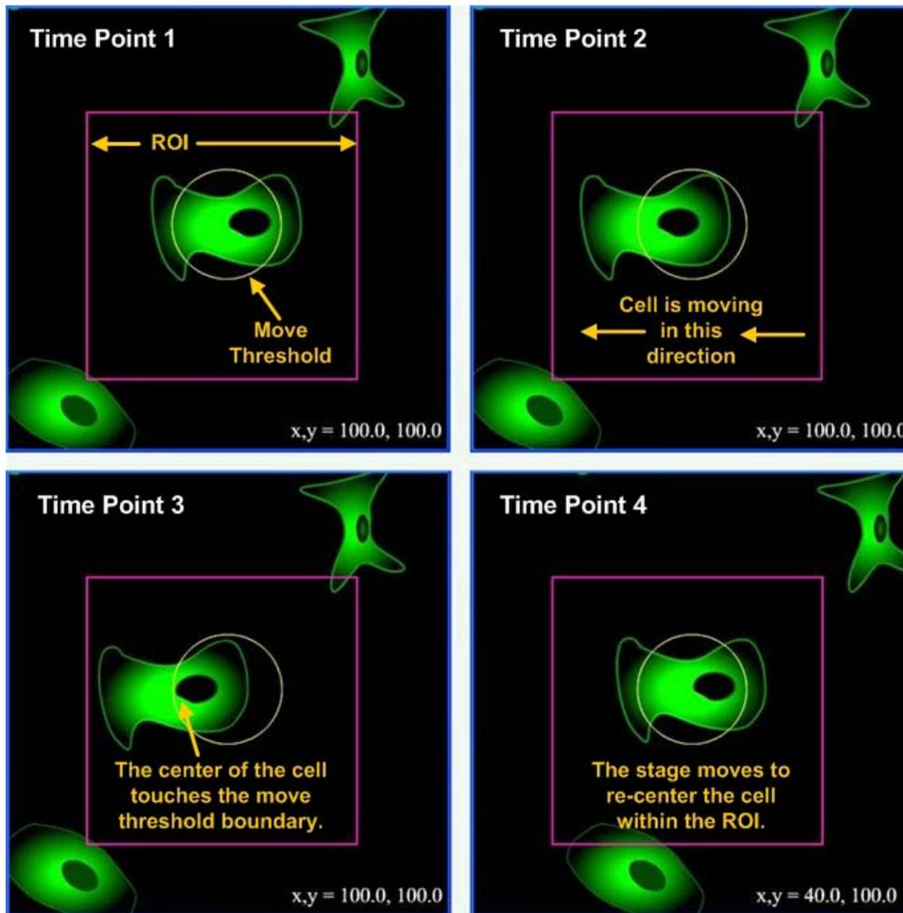
At Time Points 1 and 2, the cell is moving through the ROI (the inner square), but the center is still within the Move Threshold (the circle). At Time Point 3, once the center of the cell touches the threshold boundary, the stage moves to re-center the cell within the ROI. (Note the new stage position displayed in the lower-right corner of Time Point 4.)
