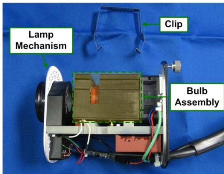
7. Lift the bulb assembly (small black box) from the two supporting pins in the lamp mechanism.
