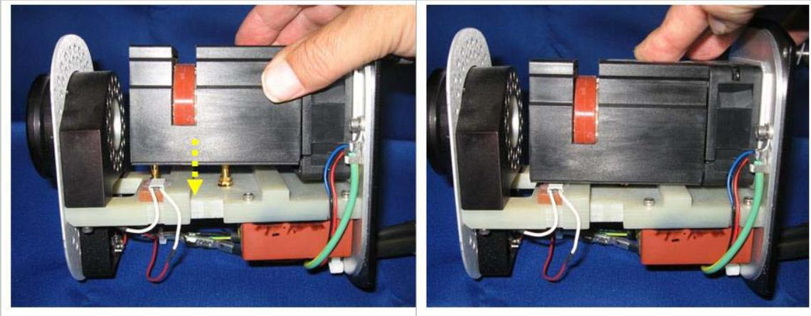
9. Replace the clip around the internal lamp assembly, making sure the clip is properly oriented.
