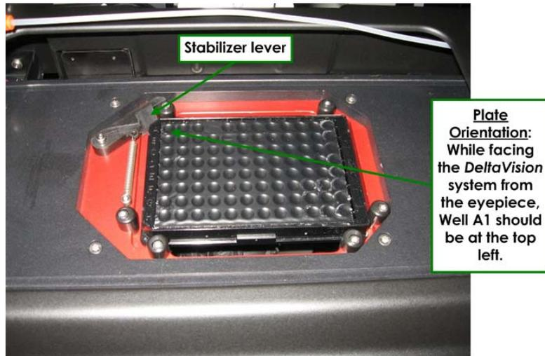
3. When loaded properly, the microtiter plate should be level in the plate carrier.
