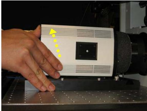
3. On the Emission filter wheel motor, disconnect the cable that connects the motor to the IC/MIC. Use a 3 mm hex key to loosen the set screw that holds the Emission filter wheel to the microscope.
