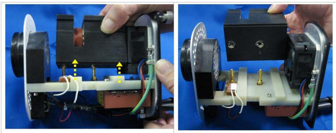
8. Replace the xenon bulb assembly with a new one (Part #34-100390-002). Insert the new bulb assembly onto the two supporting pins and press down firmly.
