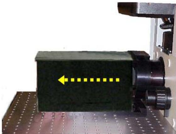
2. Remove the camera by pushing in and then pulling up on the camera end. You do not need to remove cables from the camera.
