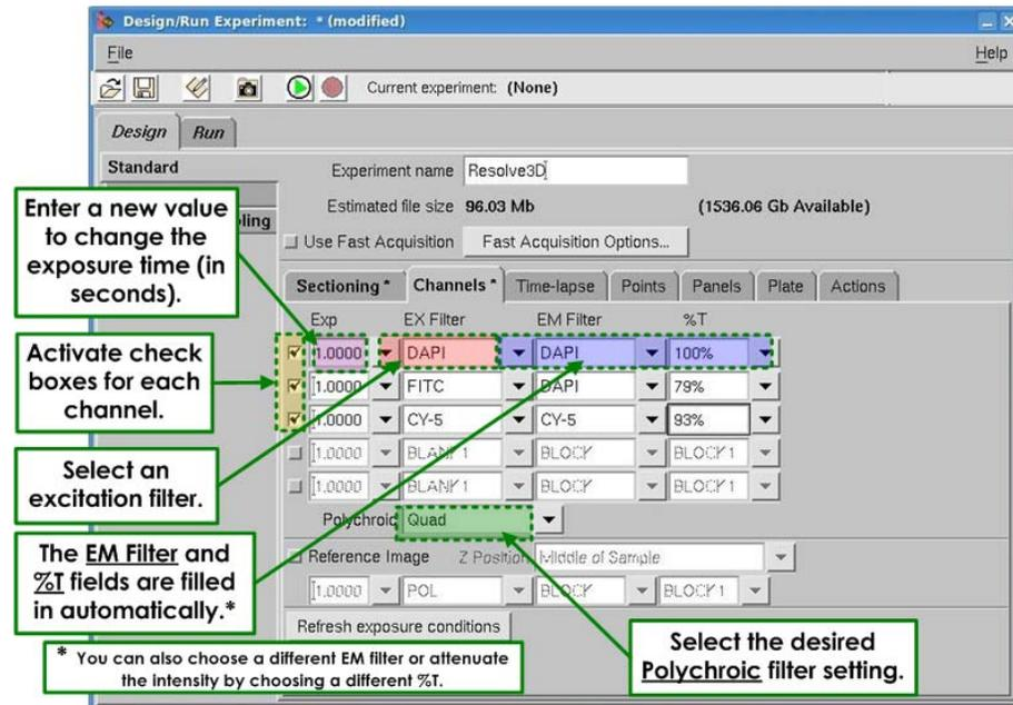
4. To change the exposure time, enter a value in the **Exp** field. Values in the **Exp** field are in seconds. For example, 0.100 is 1/10<sup>th</sup> of one second. If you do not enter a value from Resolve3D in this field, the most recently selected exposure value is automatically set for each filter.
