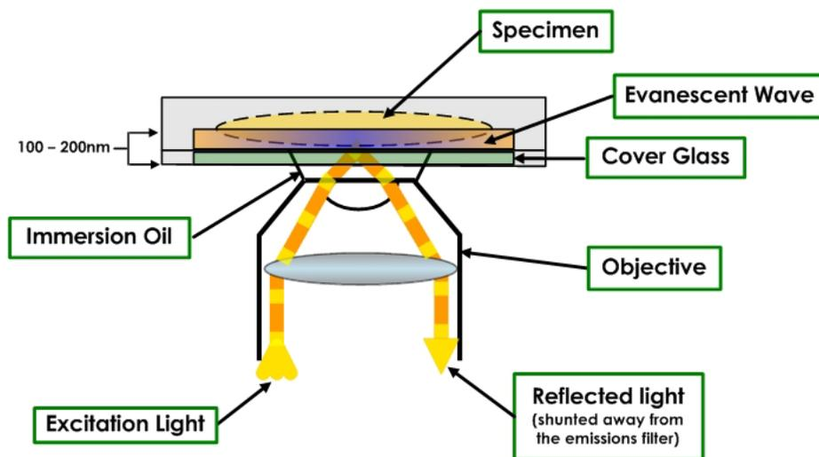
If there are fluorescent molecules in close proximity to the interface, and these molecules are capable of absorbing the wavelength of the evanescent wave, then these molecules (known as *fluorophores*) will become excited and fluoresce. Since the evanescent wave decays rapidly, molecules that are more than about 200nm from the surface of the interface will not be sufficiently excited to fluoresce. These molecules contribute to neither the signal nor the background (noise) fluorescence.
