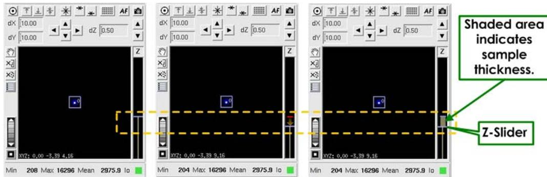
Use the Z slider to find the top and bottom of a sample. The sample thickness is indicated by the shaded area on the Z slider (shown in the image on the right).
