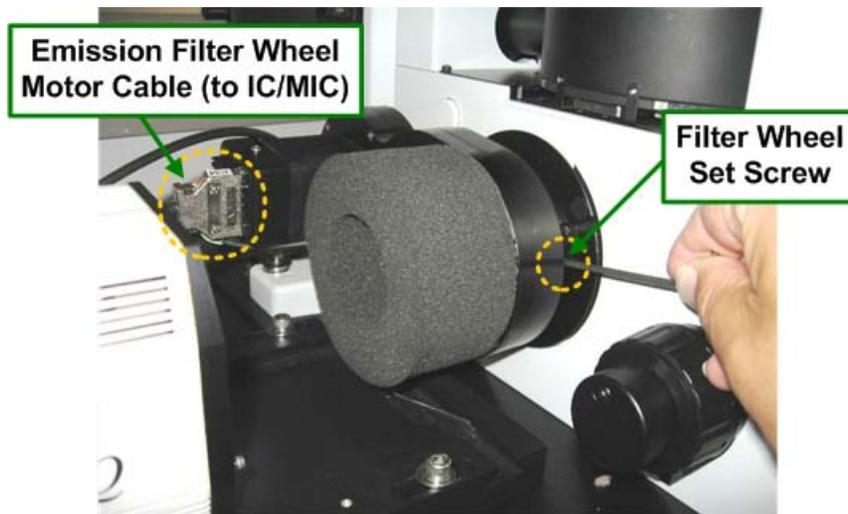
4. Remove the Emission filter wheel.
