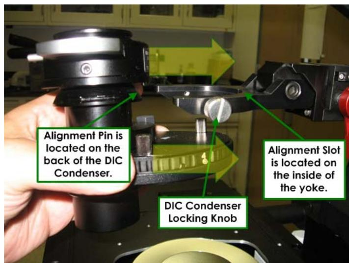
2. Tighten the locking knob on the right to fix the condenser in place.
