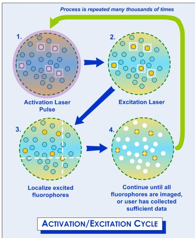
The results of a localization experiment are single-z (2D) time-lapse DeltaVision files (i.e. a movie) where each file contains the reporter images collected after a specific activation pulse.
