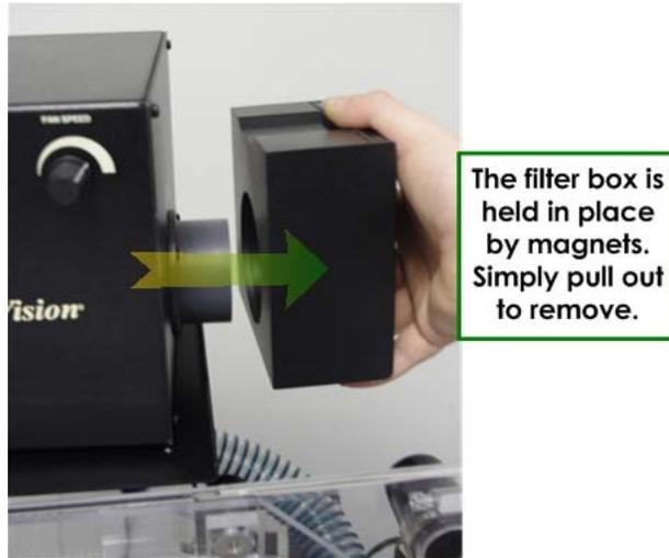
**Removing the Filter Housing**
