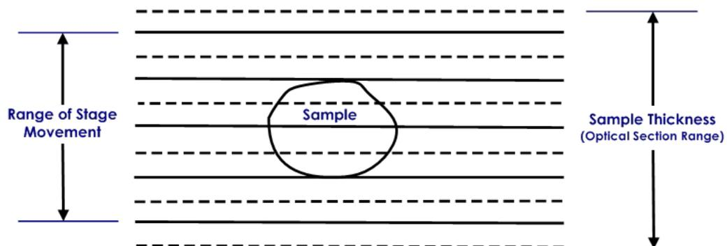
For optimal deconvolution, the Z sections should extend beyond the volume of interest by 1-3 sections.
