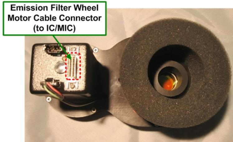
5. Install the alternate Emission filter wheel. Tighten the Emission filter wheel set screw and connect the cable from the IC/MIC to the new Emission filter wheel.
