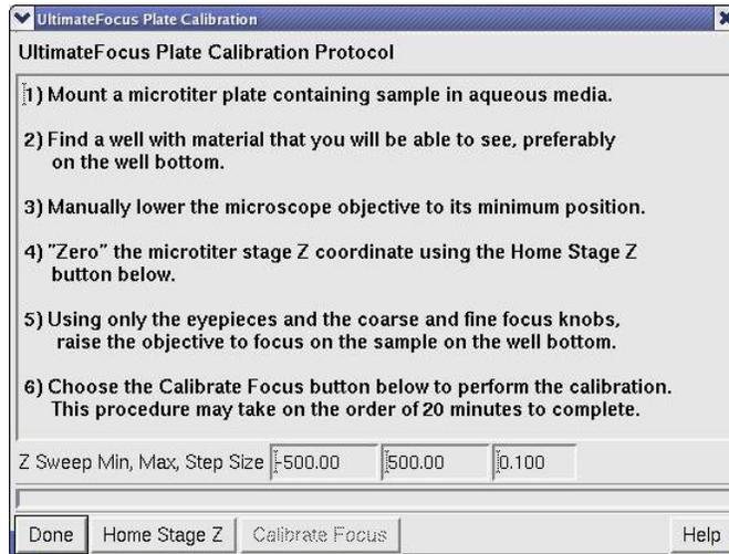
This window provides a procedure for plate calibration. The **Home Stage Z** and the **Calibrate Focus** buttons at the bottom of the window are used in the calibration procedure. You can also set the **Z Sweep Minimum**, the **Z Sweep Maximum**, and the **Z Step Size** from this window.
