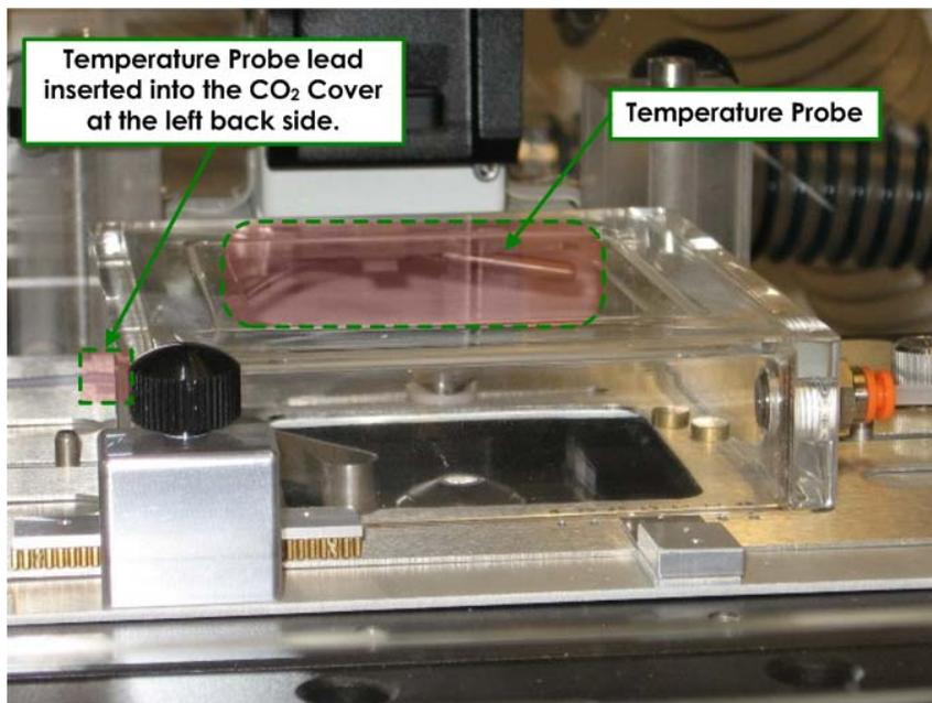
CO<sub>2</sub> Chamber - Temperature Probe
