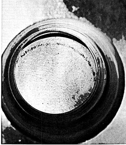
Fig. 10. Dirt on Gate of the Operational Valve.
