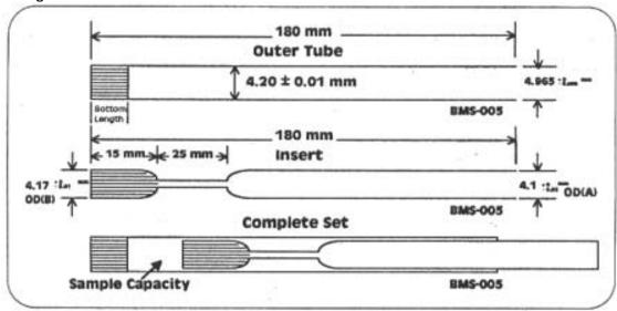
I have personally used **Shigemi tube BMS-3** with a sample volume of  $300 \square L$ . After the sample is placed into the outer tube (using a NMR pipet), the insert is pushed in all the way (slowly) till it rests on the liquid surface. There is always the likelihood of bubble formation and this can be taken care of as follows (also talk to Kirill, Hak-Jun or Murthy):
