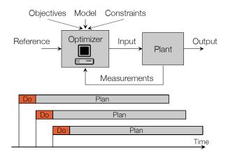
MPC: real-time, sequential optimization with constraints on states and inputs<sup>2</sup>
