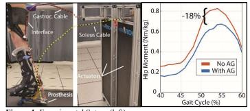
**Figure 1**: Experimental Set-up (left), Example of Prosthetic Side Hip Torque with vs. without the AG (right).
